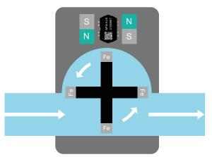
Magnets are imbedded into the rotor Ferromagnetic body is embedded into the rotor (Images for illustrative purposes and may not be mechanically accurate)
